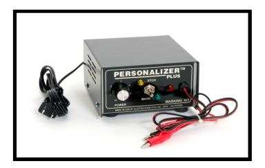
The Personalizer Plus is a very affordable medium power etching machine suitable for low volume applications. It has variable output voltage (0-20). Iow impedance. SCR phase control circuitry, and 72 watts of output power. Depths of etch of up to 0.006" can be easily achieved in most metals. In the mark (AC mode), excellent high contrast markings are produced in a just a few seconds.
